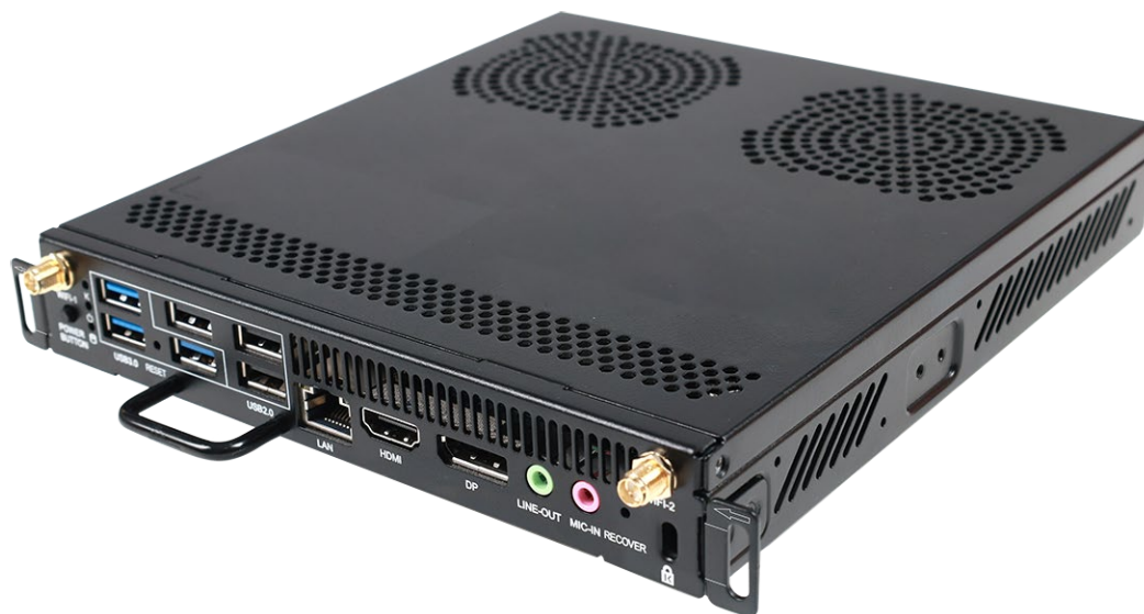
Figure 3-9 Appearance of the OPS W021 Z or OPS W022 Z
