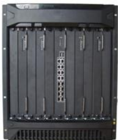
Figure 1-2 Appearance of 7U video matrix platform
