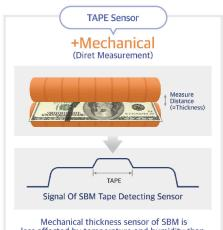
less affected by temperature and humidity than Ultrasonic thickness sensor of other companies.
