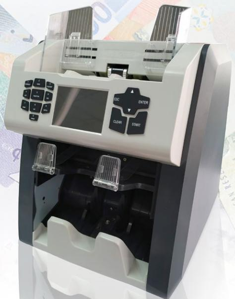
The Magner 152 banknote sorter has a modern, user-friendly interface for optimal efficiency. The Model 152 uses a full range Magnetic sensor, dual full-color RGB CIS sensors (contact image sensors), Ultraviolet transmission and sensors, as well as Infrared sensors to provide rigorous counterfeit detection and reliable performance. Up to 20 currencies are available per machine.
